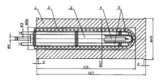
**FIGURE 2.** Thermocouples Assembly Inserted to Calibration Furnace, where:
