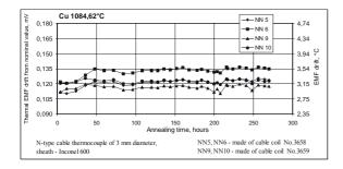
**FIGURE 4.** Thermal EMF Drift of N-Type Cable Thermocouples of 3 mm Outer Diameter Under Permanent Annealing in Air at Temperature 1085±10°C. Nominal EMF Value of N-Type Thermocouple at The Copper Freezing Point Equals to 39,502 mV.
