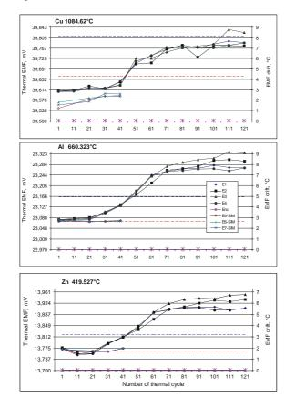
**FIGURE 3.** Thermal EMF Changes at the Freezing Points of Copper, Aluminium, Zinc for N-Type Cable Thermocouples of 3 mm Outer Diameter under Thermal Cycling in Air.
